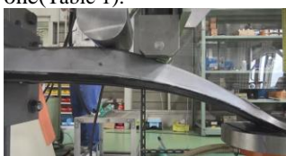
Fig. 3 patchwork B-pillar crashing device
